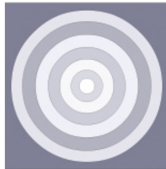
Fig. 3.18. The diffraction of light. Light brought to a focus does not come to a point, but gives rise to a blurred disc of light surrounded by several dark and light bands (the 'Airy disc').
