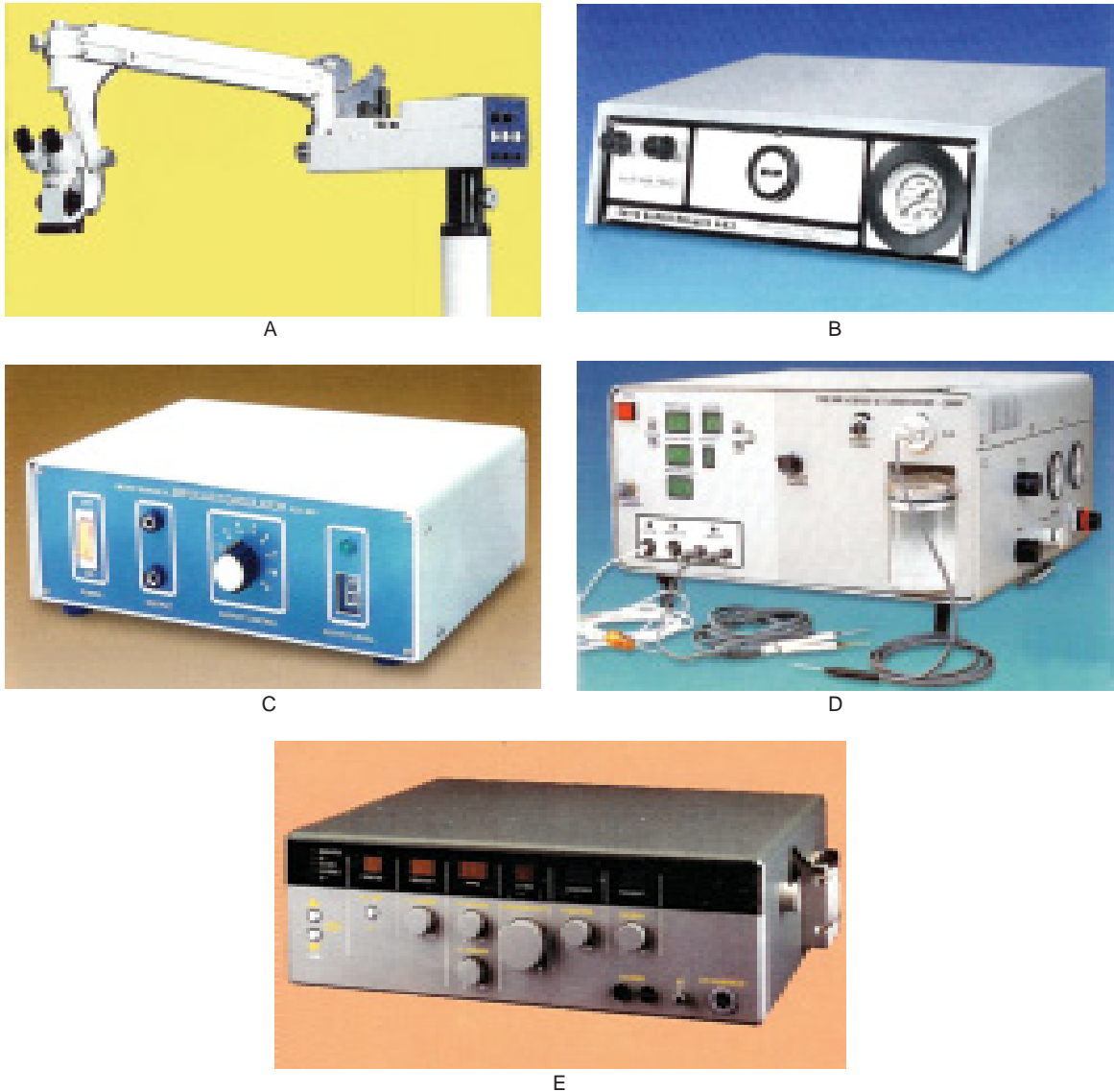
Fig. 24.5. Essential equipment for ophthalmic operation theatre: A, Operating microscope; B, Ophthalmic cryo unit; C, Wet field bipolar cautery; D, Vitrectomy unit; and E, Phacoemulsification machine.
