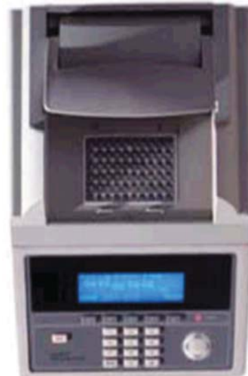
Fig. 12.6: A modern thermal cycler capable of performing 96 PCRs at a time. The model shown is ABI 9700
